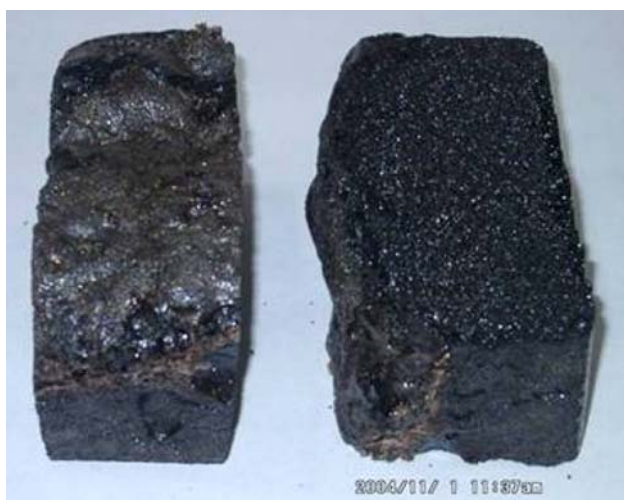
Fig. 3 Photograph of solid organic foam showing skin layer on surface and a cross-section showing uniform foam underneath the skin layer
